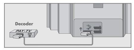
1 Connect the »AV1 « socket on the television set and the appropriate socket on the decoder using a EURO-AV cable.
