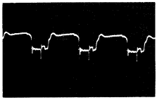
16. Q501 Base (E-PCB) Horizontal Out. 22V, 50 \mu s / Div
